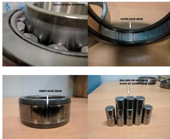
**Figure 8. Motor d.e. bearing NU316 in good condition prior the replacement (top left), bearing outer race (top right), bearing inner race (bottom left) and rolling elements (bottom right).**
